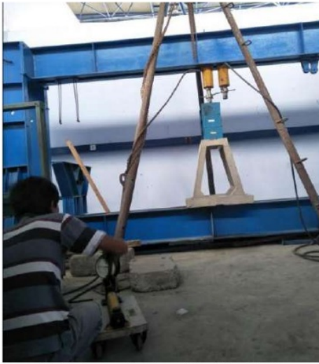
Fig.12: Pressure Test Precast Foundation Models
