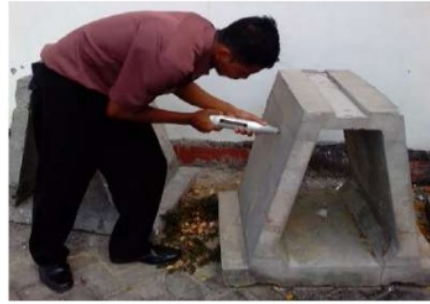
Fig. 14: Pressure Hammer Test Precast Foundation Model
