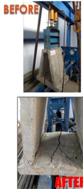
Fig. 4: Precast foundation design and pressure test [1]
