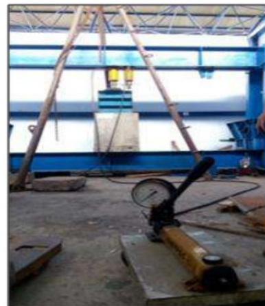
Fig.10: Test Process Tap The Foundation [2]
